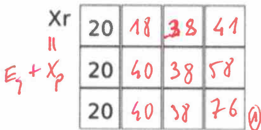
Figure 4 : Different steps of the DPCM coding of a small image.
